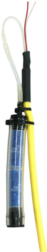
Figure 3-2: Example of New Desiccant Pack Installed on Vented Transducer Cable
