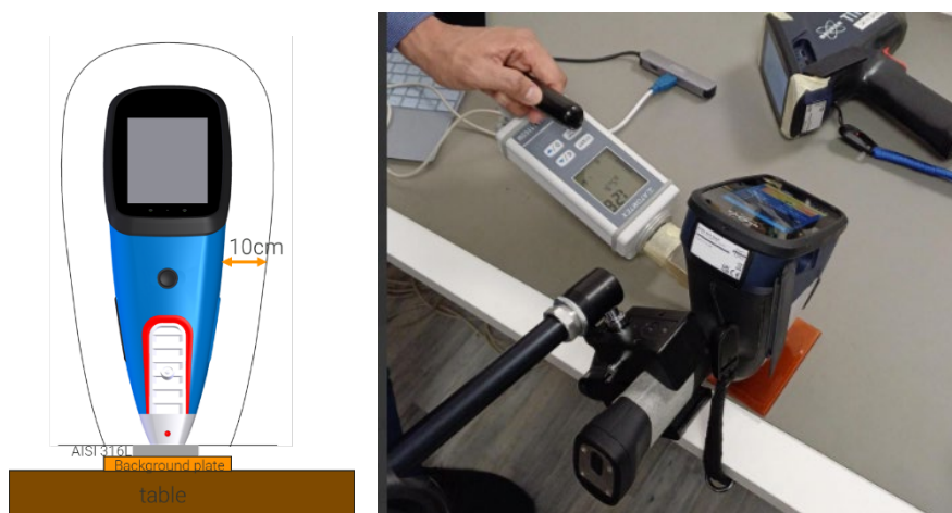
Fig. 3 Instrument in contact with the sample, background plate over the table
